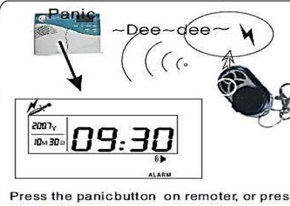
Press the panic button on remote, or press "help/bypass" key on panel for 3 seconds, and 10 seconds later the panel will dial the preset phone number. And you can disarm to cancel alarm.
