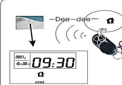
Press the key for home arm on the remote or the "HOME" key on the keypad, the panel will give voice to tell system is enter home arming. And it display home arm icon on the LCD screen.
